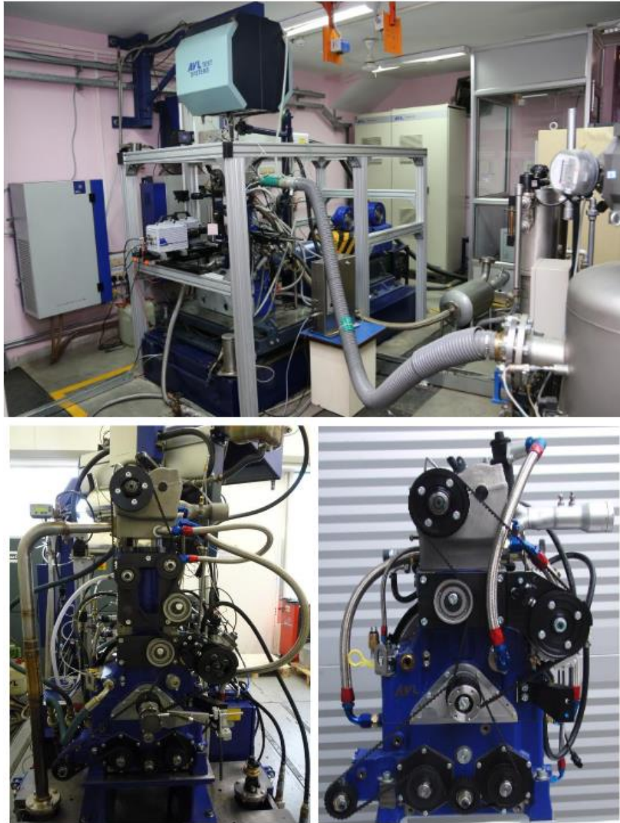
Figure #1 Single cylinder optical research engine (SCRE)
